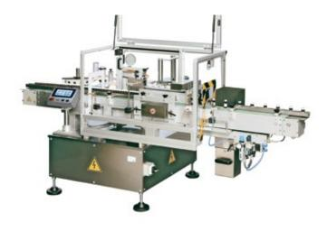
System 1 Modular is an automatic labelling system for wrap-around application on cylindrical jars and bottles: it has been as a modular unit, that can be implemented according to users needs. The basic module can be equipped with any accessory available for the labelling systems, such as print units, controls, alarms, PLCs. All functions are managed through a touch screen panel.
