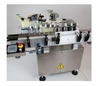
A compact and functional solution ensuring a perfect labelling of cylindrical products. The DRP device makes the product spin around during the labelling phase. A very compact body makes it fit for any environment.
