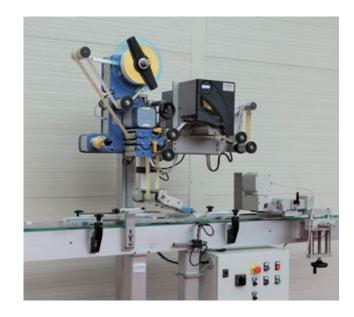
System 2 Twist applies pressure-sensitive labels on the top of every kind of products. The conveyor running at a fixed speed is the ideal solution for out-of-line applications with manual loading, while for in-line applications it can be equipped with an inverter with speed variator. Print units can be installed to print variable data, bar codes and images.
