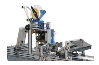
Automatic labelling system especially designed to process cards, doypack, envelopes, leaflets, flat boxes which are automatically taken from a loading stacker and conveyed horizontally by means of a vacuum conveyor system. This system is available both in the version with alternate or continuous motor and can be equipped with feeders, labellers and print units for dispensing, labelling and printing products.
