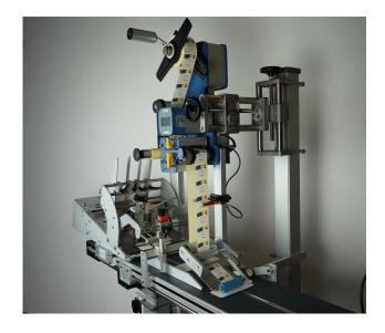
System 9 Light is a labelling system especially designed to process and label flat lying product such as envelopes, leaflets, magazines and die-cut cartones with maximum A4 size. This special configuration features the system applying radiofrequency antitheft labels within die-cut cartons.
